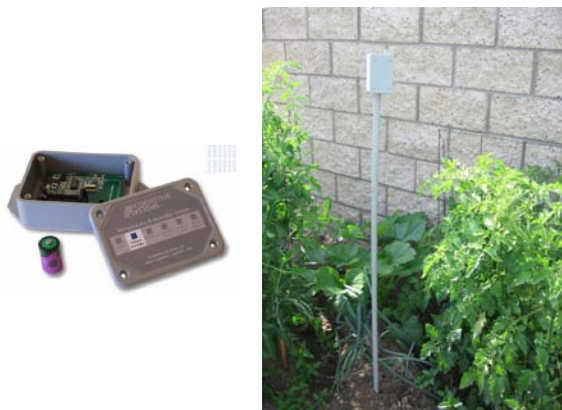
Fig. 2: WSN unit with microprocessor, transmitter, battery and built-in sensors for monitoring atmospheric temperature and humidity and wired sensors for wind speed/ direction and
