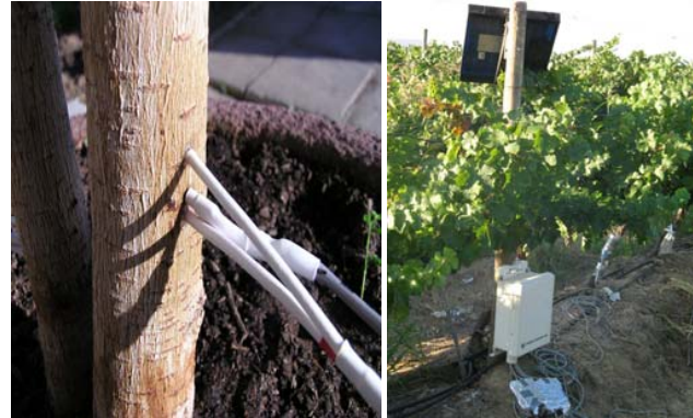
Figure 3. Measuring sap flow with HPM
