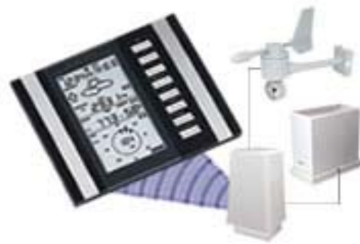
Figure 4. Wireless Telemetry Climate Data Collection Instruments and in situ Implant Sensors (La Crosse WA2300)
