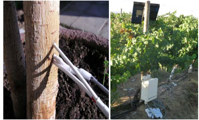
Figure 3. Measuring sap flow with HPM
